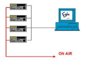
In a system with VTRs the main characteristic is that the technology is based on tape. The system is multiform, easy to maintain and it supports standard video. Unfortunately the are more negative aspects about his system than positive ones: tapes need to be frequently reloaded, commercials must be previously prepared and it's very difficult to maintain video quality. The system has a low MTBF and it is not fault tolerant.
