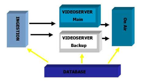
With ETERE Automation, you can manage a Backup system without any effort. Two systems are seen by operators as a single videoserver. The Backup system comes automatically into operation, and it's autonomously updated by Etere Media Manager.
