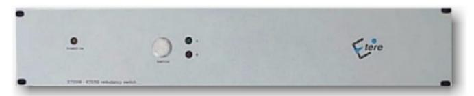
The device is bi-directional, data are send from 1 to 2 and from 2 to 1. ETERE Redundancy Switch does not add noise nor modifies the signal to be switched, the switching is relay controlled. Lines are independent from one another, the protocol of each serial line can differ from the others. The switching can be manual from the front panel or remote controlled by GPI from ETERE clone.
