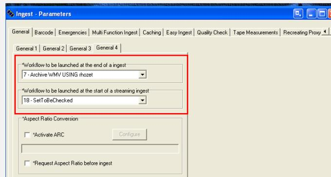
The image below illustrates how Etere allows setting the workflow to be launched at the start and end of an ingest process to for example, **create a low resolution** version or **normalize the audio** of captured contents:
