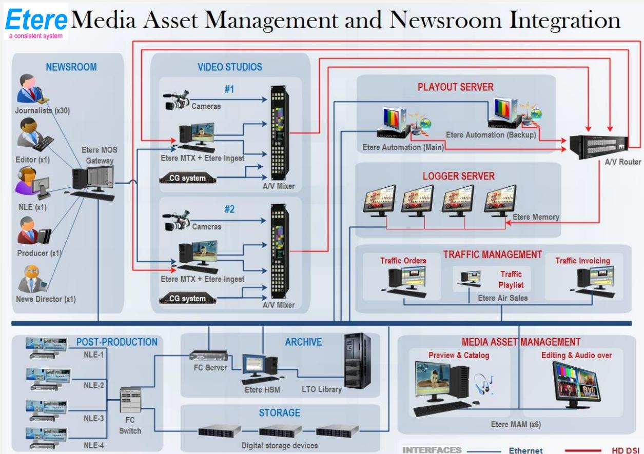
The solution proposed by Etere will provide the station with a rock-solid distributed system able to integrate into a single solution the key features of a Media Asset Management system empowered with a Traffic service for commercial assets, plus a tight integration with the Newsroom Computer System used by the station. Additionally, Etere’s solution will permit to straightly connect ingest channels with Etere MAM to browse and edit media assets before their delivery.
