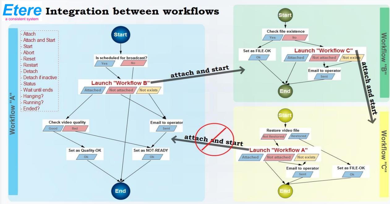
As shown above, for example, if 'workflow A' calls 'workflow B' and the 'workflow B' calls 'workflow C', the 'workflow C' will not be able to call the 'Workflow A'.
