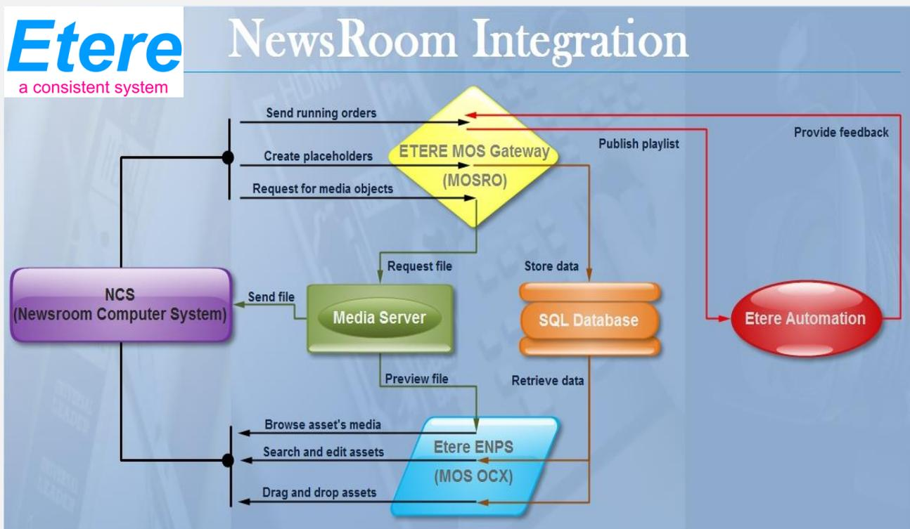
The diagram above illustrates how Etere provides an integrated two-way interface to newsrooms systems using the following modules:
