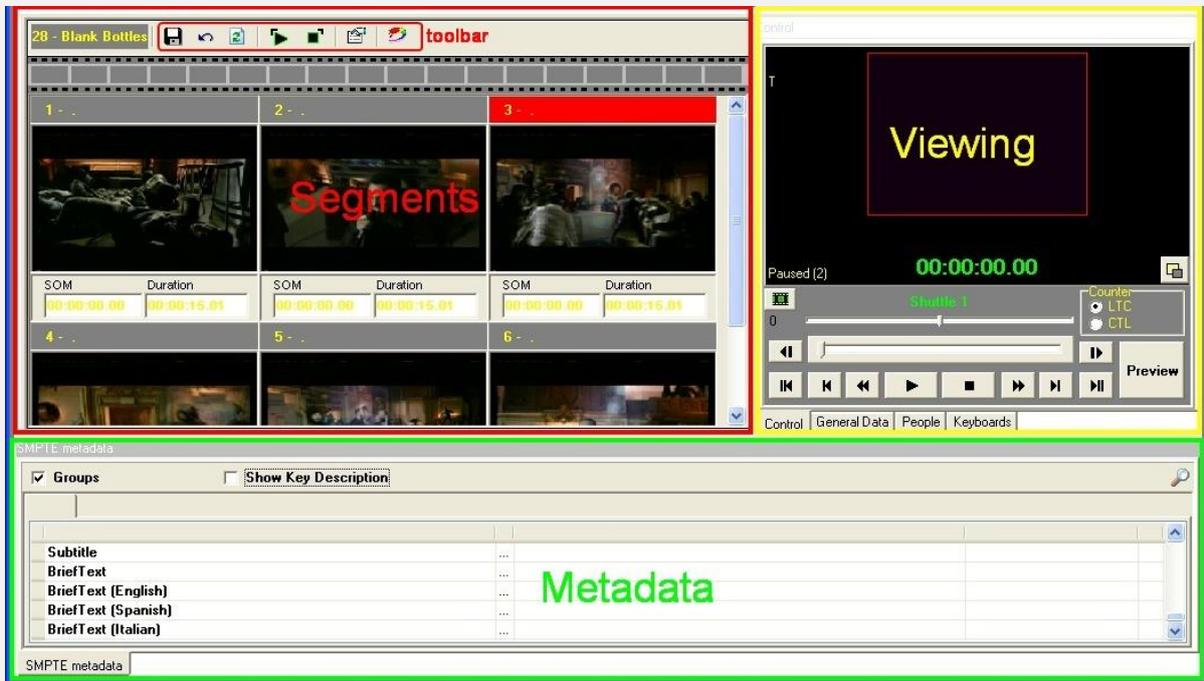
Etere also allows restoring only a part of video files by creating either high or low resolution video files including specific segments described on the source video EDL, it is important to note that as usual on Etere's operations, the conforming of video files is fully performed via workflow:
