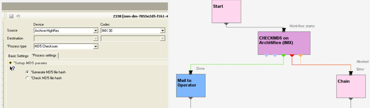
The workflow editor allows creating custom Checksum workflows to either generate or check the MD5 hash status of a video file.
