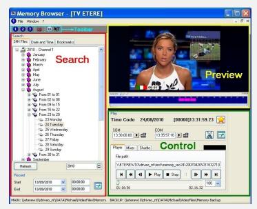
Etere Memory allows recording and viewing clips at the same time with just a few frames of delay while offering the following key features:
