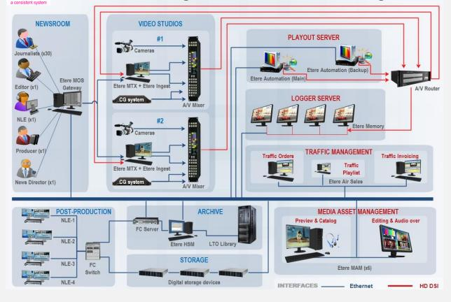
The solution proposed by Etere will provide the station with a rock-solid distributed system able to integrate into a single solution the key features of a Media Asset Management system empowered with a Traffic service for commercial assets, plus a tight integration with the Newsroom Computer System used by the station. Additionally, Etere's solution will permit to straightly connect ingest channels with Etere MAM to browse and edit media assets before their delivery.
