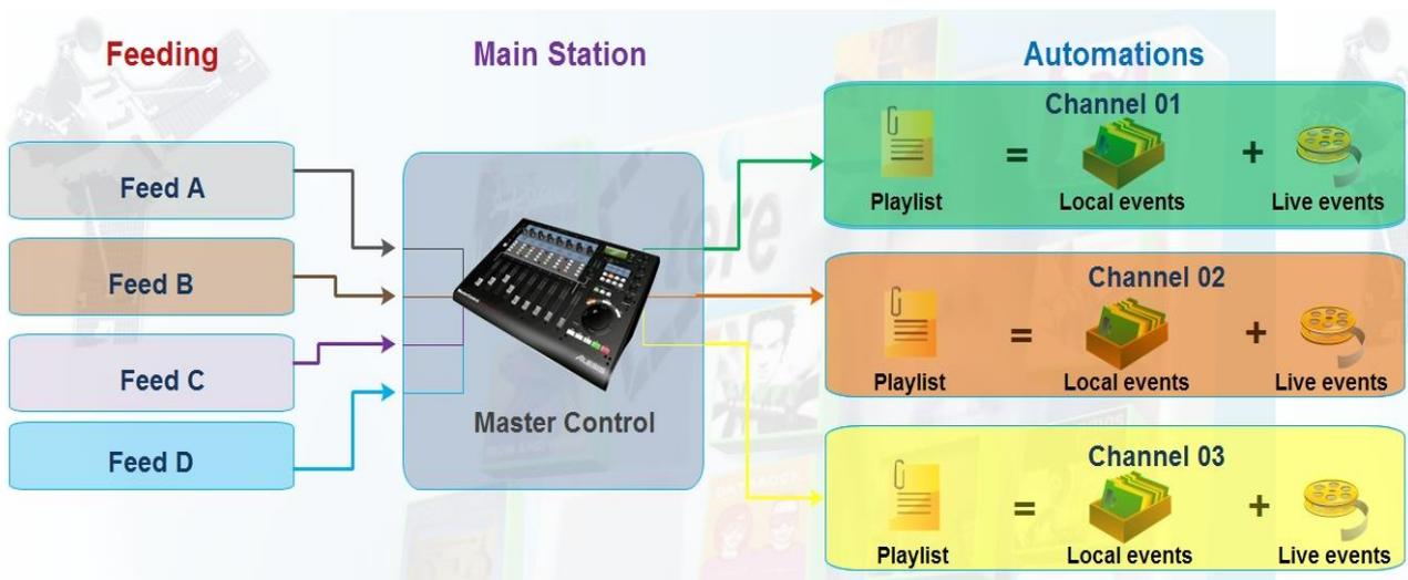
The master control will be located in the main facility, and will go live on local time. Each automation channel will send on air a schedule composed by events locally scheduled and live events arriving from the main station.
