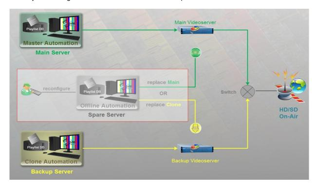
As shown in the diagram above, software automations and hardware servers involved in the playout system will be referenced in the following text using the following names:
